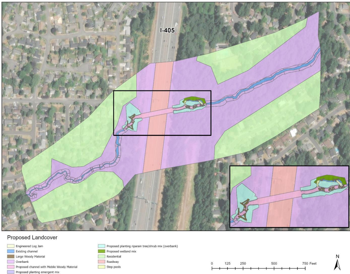
Figure 5-5: Spatial distribution of proposed conditions roughness regions in SRH-2D model
